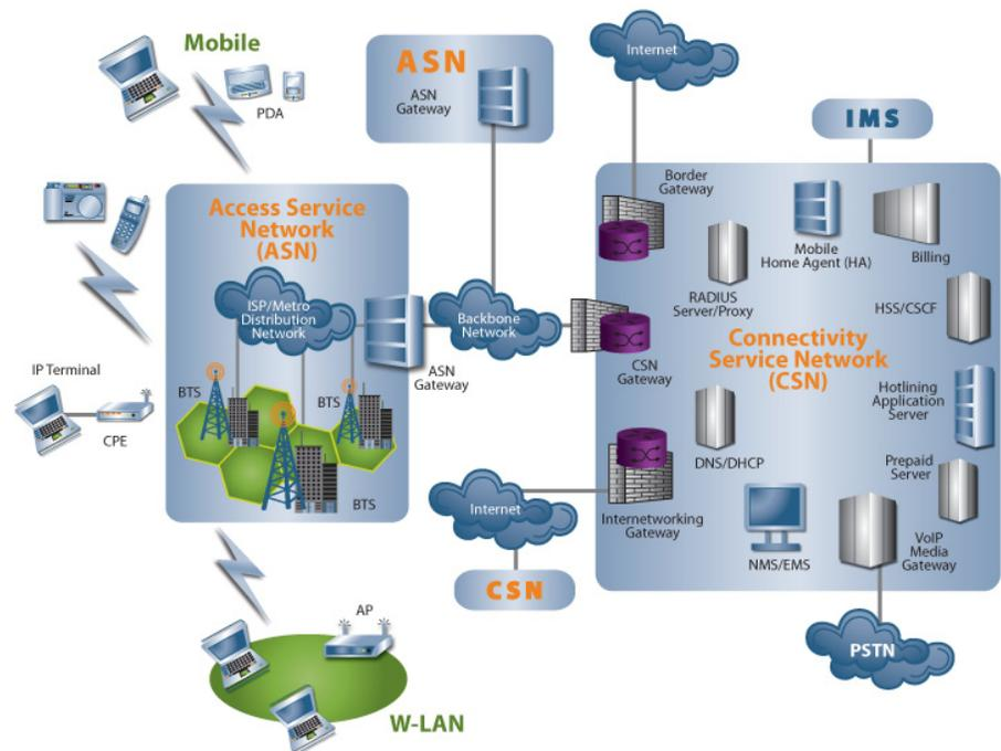
Figure 3. Traditional WiMAX Core Network Architecture
