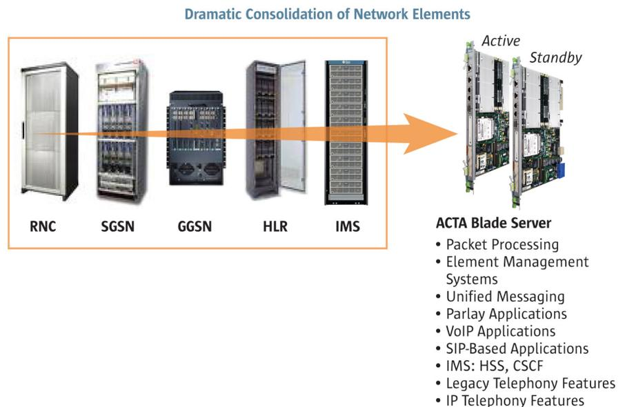
Figure 1. Consolidating Network Elements with the Sun™ Unified Network Platform
